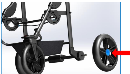
Fig. 12 Removal and installation of rear wheels
